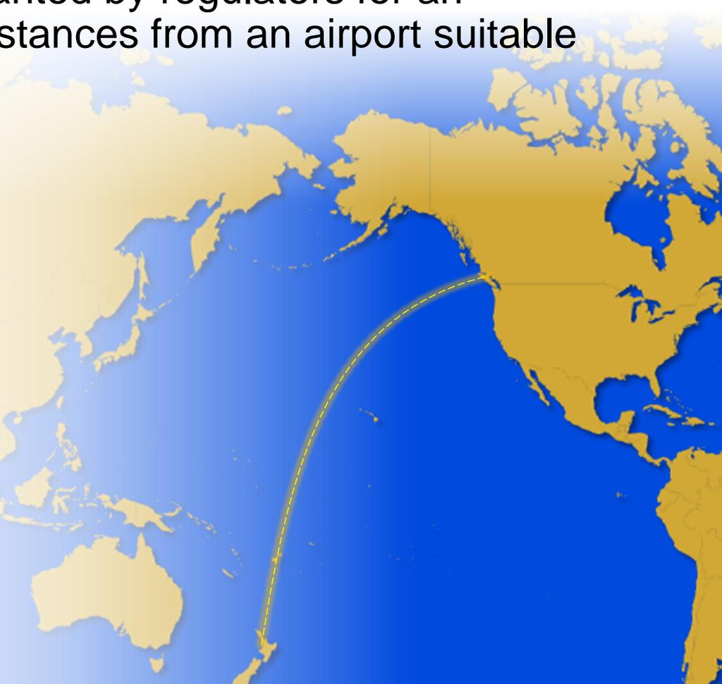
**ETOPS Enables More Direct and Efficient Routing**
